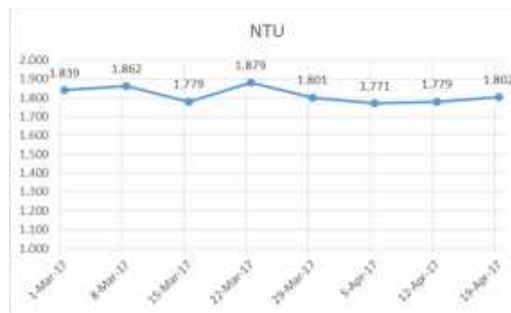
Gambar.1 NTU aktual Cooling Tower
