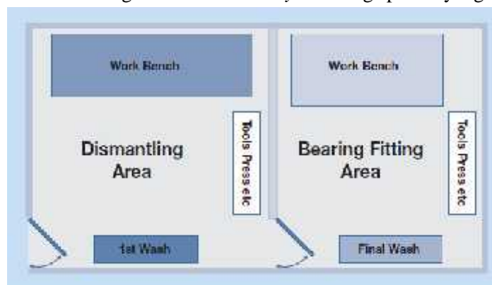
Gambar 8 Layout Ruang Spindle yang Ideal (Sumber : NSK Machine Tool Spindle Bearing Selection & Mounting Guide)
