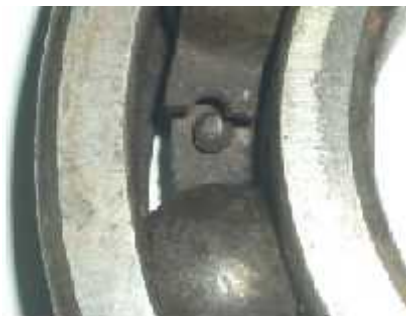
Gambar 3.10 Cage Bearing Patah
