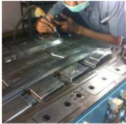
“Gambar.6 Dinding Hole Digerinda”
